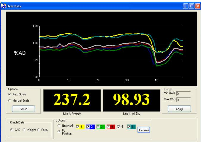
The last 300 bales are displayed by drop position. This allows the user to view trends in moisture or weight both horizontally and vertically across the pulp web.
